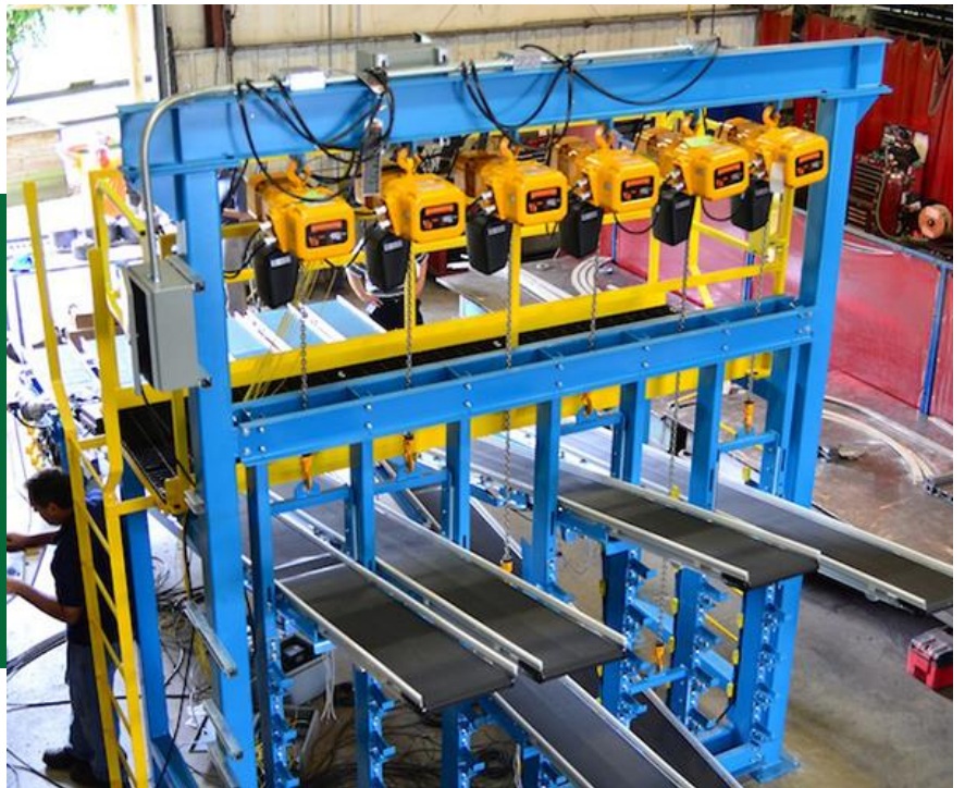
Off Site Pre-Installation Testing of Hinged Belt System
